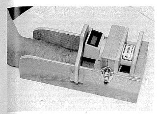
FIG. 1. Hand-arm receptacle housing a dynamometer that was used to measure isometric wrist extensor strength.
